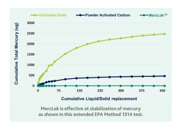
These results have been confirmed in numerous batch-reactor and column studies across a range of soils and waste materials and demonstrates **MercLok's strong efficacy to capture and immobilize mercury.**
