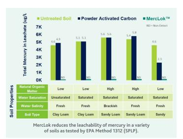
Results from soil studies using industry accepted testing methods have demonstrated MercLok's ability to capture elemental, ionic, and methylmercury in soil and reduce the leachability of mercury by greater than 95%.
